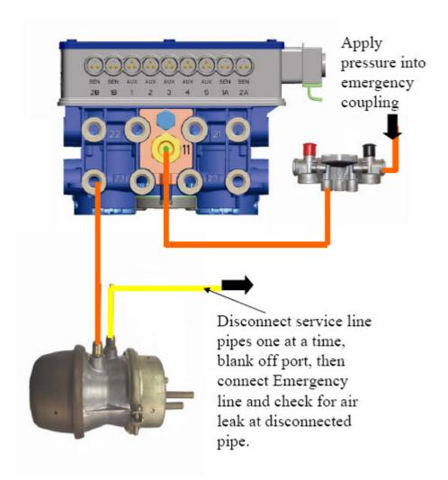
If the truck is not available then you will need to regulate the red line pressure through a range from approx 6.0B to 9.0B in 0.5B increments as it may be the case that the chambers only leak at a certain pressure.
