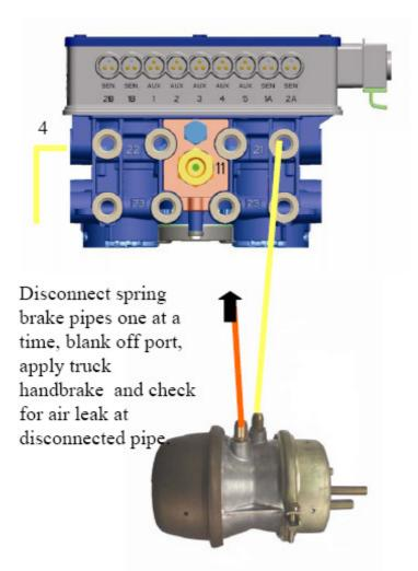
If the truck is not available then you will need to regulate the yellow line pressure through a range from approx 6.0B to 9.0B in 0.5B increments as it may be the case that the chambers only leak at a certain pressure.
