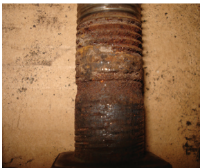
Corroded wheel stud
