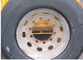
Wheels cleaned and in a serviceable condition for fitment
