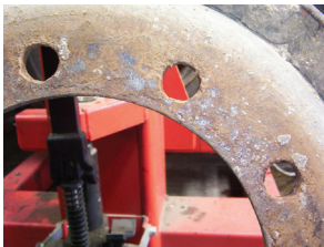
Debris trapped between wheels
