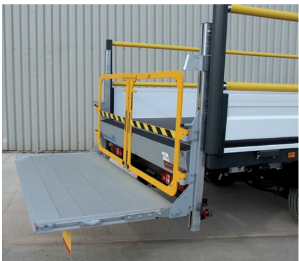
Typical example of column lift with runner mounted 3 position gates
