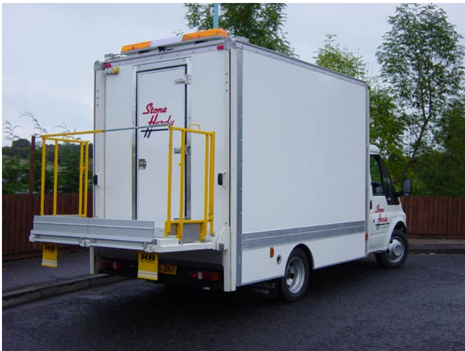
Typical example of a column lift with 3 sided fall protection and 3 way folding ramps
