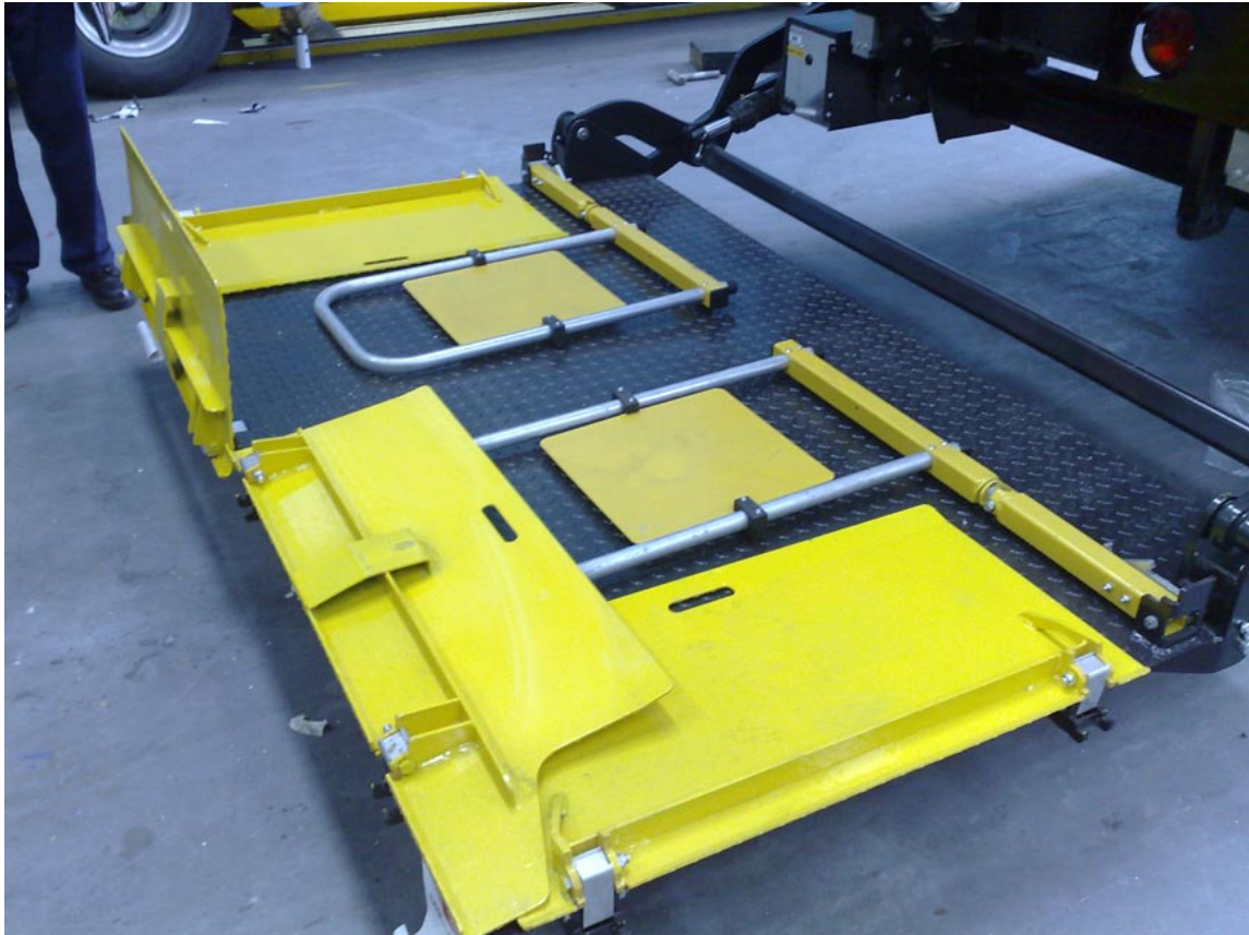
Typical example of a slide away tail lift with folding 'p' gates and 3 way folding ramps
