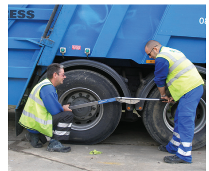
Physical use of a torque wrench
