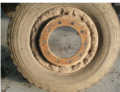
Severely dirt-contaminated wheel rim
