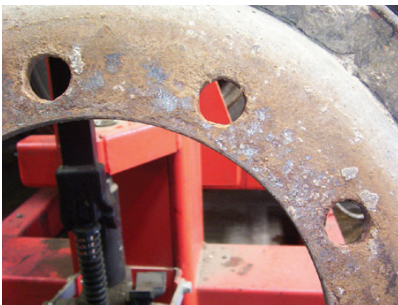
Debris trapped between wheels
