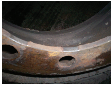
Worn wheel centre bore spigot
